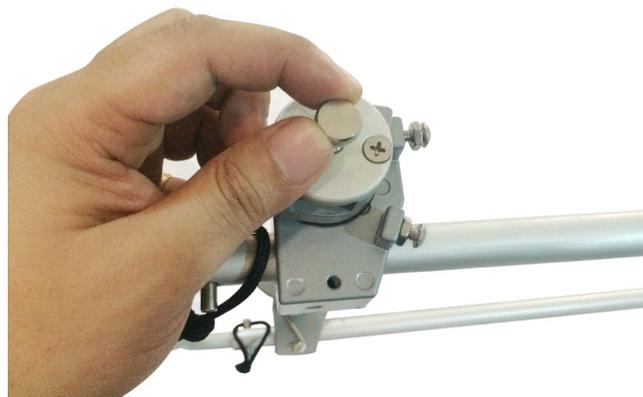
3.2. Loosen wheel bar thumbscrew on pivot assembly (A).
