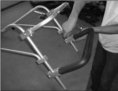
2.3 Hold the connector block screw steady with an open-end wrench while securing the clip connector screw with a hex wrench.
