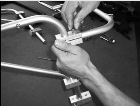
1.3 Place the connector block screw and the clip connector screw together inside the upper crossbar connector block.
